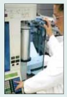
Surface areas of MgSt and other pharmaceutical ingredients are measured by gas adsorption at cryogenic temperatures. The NOVAe series from Quantachrome features multiple sample capability and optional IQ/QQ/PQ & 21CFR Part 11 compliance packages.
