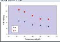
Two brands of MgSt show similar trends in surface area loss as function of increasing degas temp.
