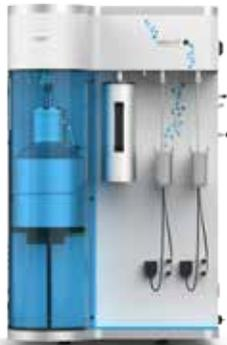
Due to their ability to characterize extremely small pores, these instruments assist in battery separator design efforts, since they facilitate the accurate assessment of pores present in sizes as small as 0.35 nm.
