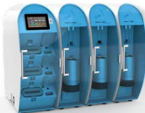
Figure 2. AutoFlow BET+ ® with Three Modular Analysis Stations.
